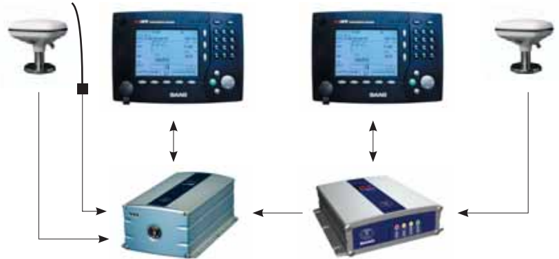
Combined AIS and DGPS System
