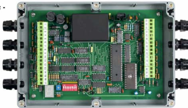
Model NT920 HDI ~ typically for use with electronic / GPS compass types and/or pulse output speed logs.
