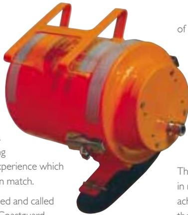
of onboard activity, including audio (both speech and ambient sound), radar, time, position, speed, heading, telegraph demand, engine and propeller activity, as well as a host of additional information.
